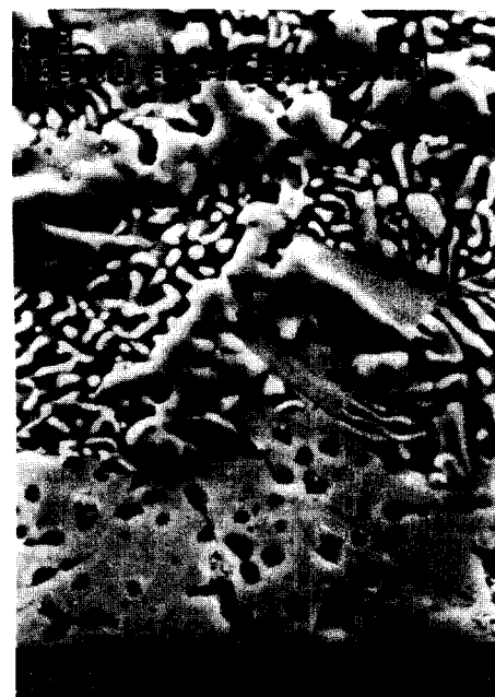
Figure 2 Interaction region of a heat treated plasma sprayed Y-Ba-Cu-O coating on a Ni-Cr bond layer (see text for details)
