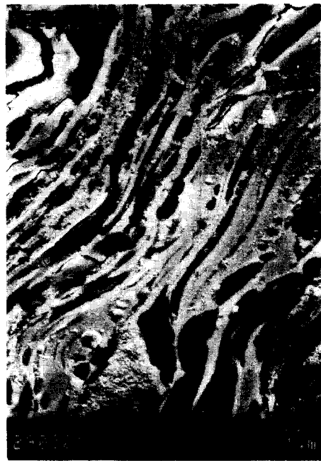
Figure 1 Lamellar structure of an as-deposited plasma sprayed Y-Ba-Cu-O coating
