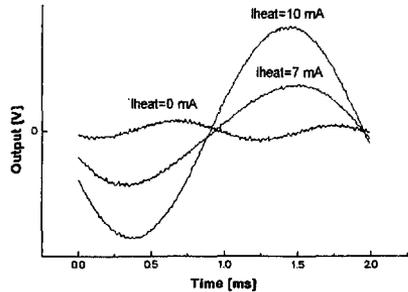
Fig. 13. Response of the combination of the  $\mu$ -flow and measuring electronics as a function of the heater current in a heater sensor configuration. The sensor current was 10 mA.
