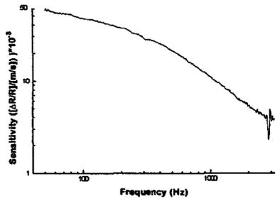
Fig. 8. Sensitivity of the  $\mu$ -flown. The shs configuration was used. The sensor and heater current were each 10 mA.
