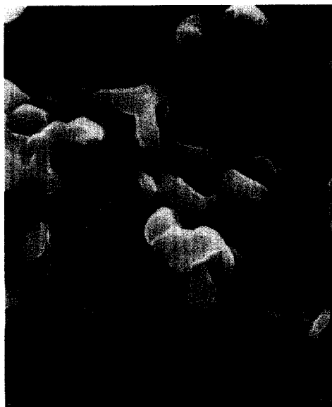
Fig. 9. SEM of La 0.6 Sr 0.4 Co 0.8 Fe 0.2 O 3 surface showing decomposition.
