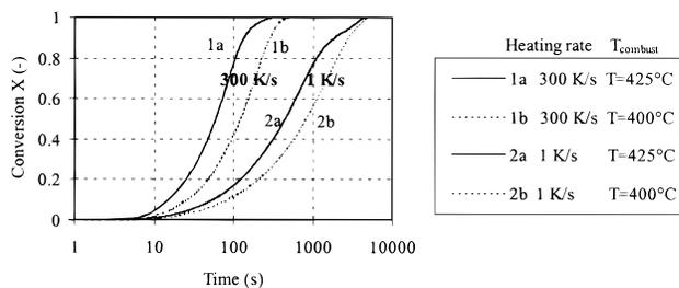
**Figure 4.** Influence of the heating rate on the burn-off curve (recorded for the packed-bed reactor at an oxygen concentration of 18 vol %). Char preparation conditions: pyrolysis temperature, 600 °C; holding time at 300 K/s, 60 s; holding time at 1 K/s, 375 s.
