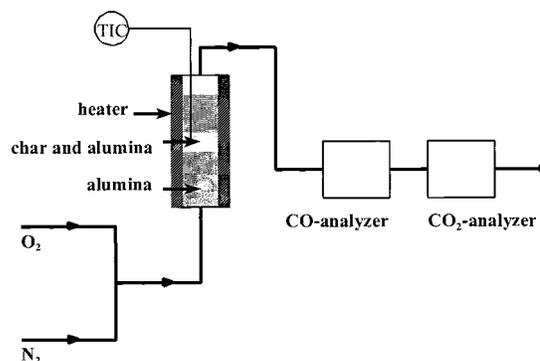
**Figure 2.** Flow sheet of the packed-bed equipment.
