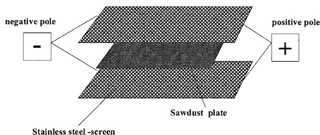
**Figure 1.** Schematic picture of the screen heater reactor.
