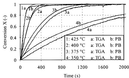
**Figure 7.** Comparison between TGA and packed-bed experiments (18 vol % O<sub>2</sub>) in a conversion versus time plot and for different combustion temperatures.
