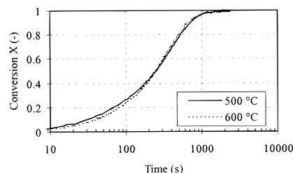
**Figure 5.** Influence of the pyrolysis temperature on the char burn-off curve (recorded for the TGA at a combustion temperature of 300 °C and an oxygen concentration of 18 vol %). Char preparation conditions: heating rate, 300 K/s; pyrolysis time, 20 s.
