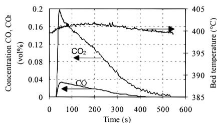
**Figure 3.** Time-dependent CO<sub>2</sub>, CO, and temperature profiles during a packed-bed combustion experiment.
