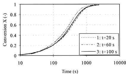
**Figure 6.** Influence of the pyrolysis time on the char burn-off curve (recorded for the TGA at a combustion temperature of 300 °C and an oxygen concentration of 18 vol %). Char preparation conditions: heating rate, 300 K/s; pyrolysis temperature, 600 °C.
