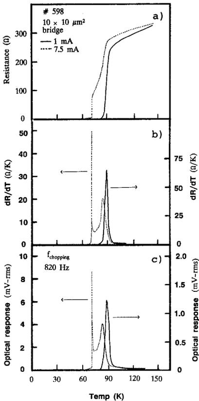
Fig. 4. The resistance  $R$  (a), its thermal derivative  $dR/dT$  (b), and the optical response (c) of bridge #598 as a function of temperature at a bias current of 1 and 7.5 mA.
