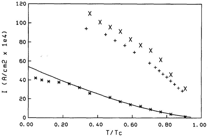
Fig. 6. Critical current as a function of  $T/T_c$  for a  $10 \times 10 \mu\text{m}^2$  bridge. Experiment: "\*"  $I_{c0}$  of bridge No. 598-2, "+"  $I_s^*$  of bridge No. 598-1, "x"  $I_s^*$  of bridge No. 597-1. Theory: solid line, fit assuming  $I_{c0} \propto (1 - T/T_c)^{3/2}$ .
