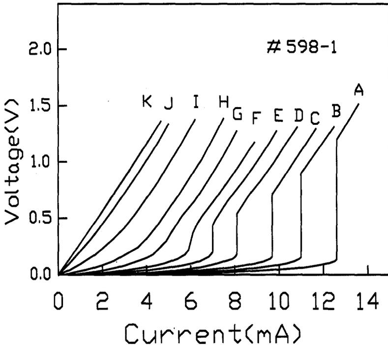
Fig. 3. A set of VCCs of a  $10 \times 10 \mu\text{m}^2$  bridge (sample 598-1) at different temperatures: A: 73 K, B: 75 K, C: 77 K, D: 79 K, E: 81 K, F: 83 K, G: 85 K, H: 87 K, I: 89 K, J: 91 K, and K: 93 K; at the voltage step region only the branch with increasing current is given.
