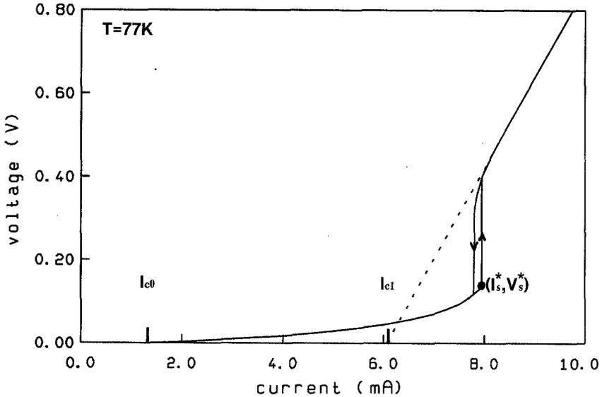
Fig. 2. A VCC of a  $10 \times 10 \mu\text{m}^2$  bridge (sample No. 597-1) at 77 K. Arrows identify the two branches of the voltage step region.
