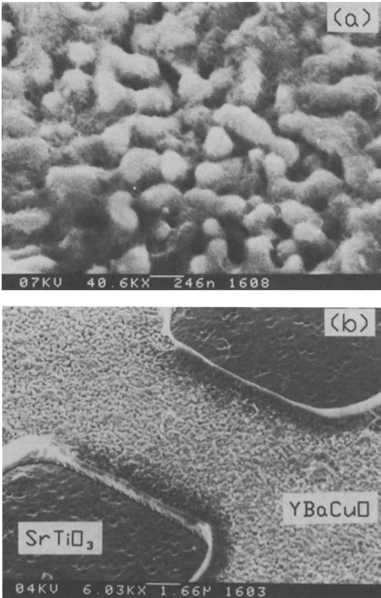
Fig. 1. SEM picture of our highly granular YBaCuO thin film made by aerosol deposition on a SrTiO<sub>3</sub> substrate (after heat treatment). (a) detail with large magnification (bar indicates 246 nm). (b) view of a  $10 \times 10 \mu\text{m}^2$  microbridge made by ion-beam milling from the same film as in (a) (bar indicates 1.66  $\mu\text{m}$ ).
