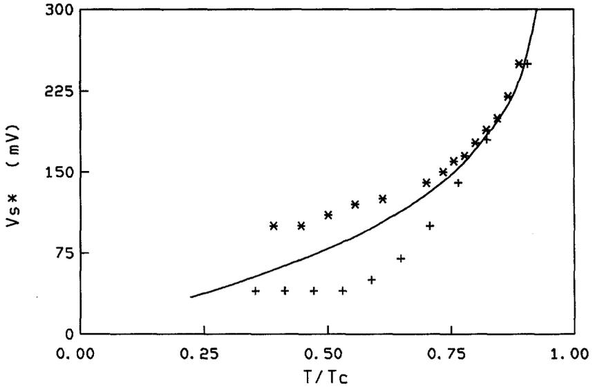
Fig. 5. The voltage  $V_s^*$  as a function of  $T/T_c$  for a  $10 \times 10 \mu\text{m}^2$  bridge. Experiment: "+" bridge No. 597-1; "\*" bridge No. 598-1. Theory: solid line, fit according to Eq. (3).
