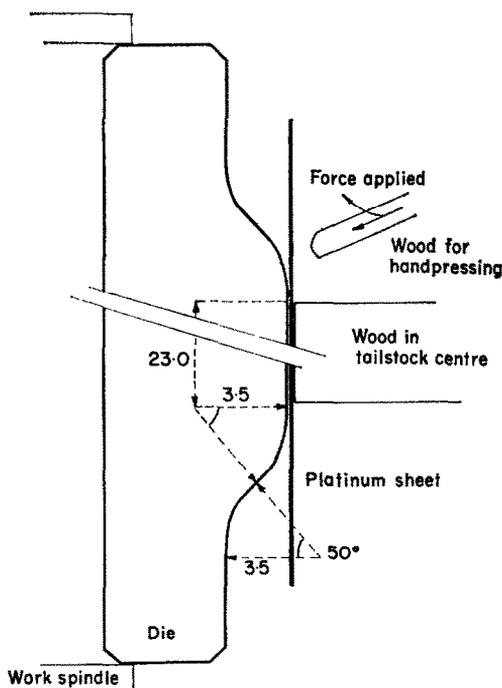
FIG. 1.—Form of the die and arrangement for the forming process.
