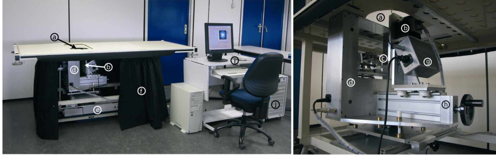
Fig. 1. The Twente Photoacoustic Mammoscope. a – aperture to insert breast, b – ultrasound detector matrix, c – glass window of d – scanning system compartment, e – Q-switched Nd:YAG laser operated at 1064 nm with 5 ns pulses, f – laser safety curtain which is drawn around the instrument during the measurement, g – interface electronics between detector and computer, h – linear stage carrying detector matrix driven by handwheel to apply mild compression to breast, I – laser remote control unit, j – laser power supply.
