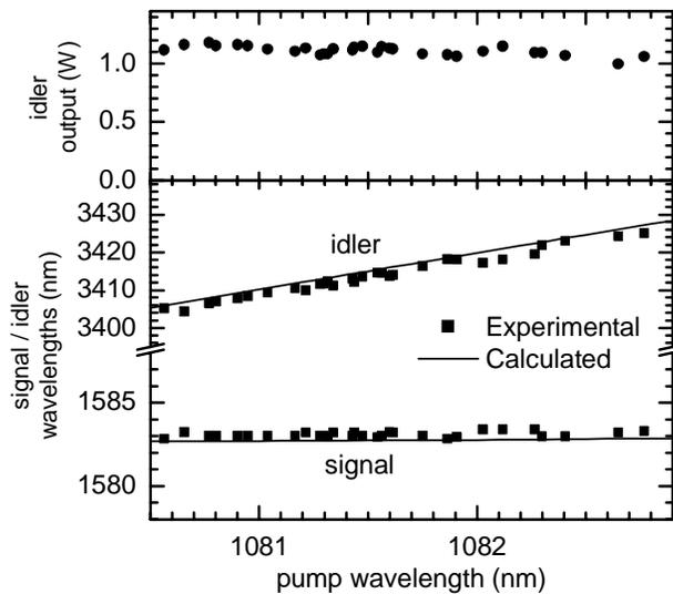
Fig. 2. Variation of OPO output wavelengths (lower plot), and corresponding idler output power (upper plot), during pump tuning by seed laser DBR section alone. PPLN grating period was 29.75  $\mu\text{m}$  and temperature was  $180.5^\circ\text{C}$ . Calculated tuning data was derived using the Sellmeier equations of Jundt [10].
