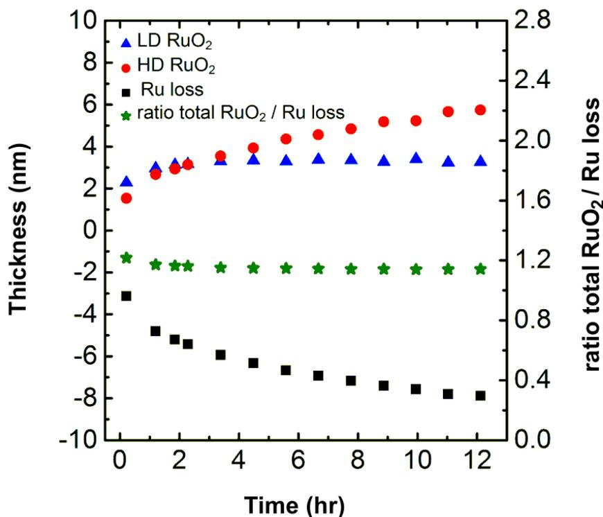
FIG. 2. (Color online) Left-axis: RuO<sub>2</sub> thickness and Ru loss as a function of annealing time for 400°C. Low density (LD) RuO<sub>2</sub> thickness (triangles), high density (HD) RuO<sub>2</sub> thickness (circles) and Ru loss (squares) are plotted. Right-axis: ratio between total RuO<sub>2</sub> formed (summed low density and high density) and Ru loss as a function of annealing time for 400°C (stars). The layer thicknesses were determined with the accuracy of  $\pm 0.1$  nm.
