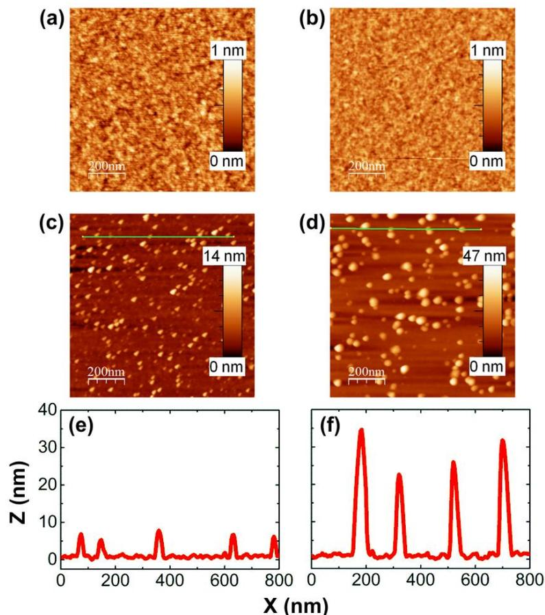
FIG. 3. (Color online) Atomic force microscopy (AFM) images ( $1 \times 1 \mu\text{m}$ ) of the as deposited (a), and 20 minutes annealed samples at  $175^\circ\text{C}$  (b),  $200^\circ\text{C}$  (c), and  $300^\circ\text{C}$  (d). Line profiles of the 20 minutes annealed samples at  $200^\circ\text{C}$  (e), and  $300^\circ\text{C}$  (f), are represented by the straight lines shown in the AFM images (c) and (d), respectively.
