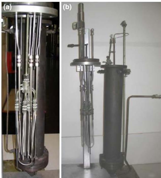
**Fig. 2** Pictures of the membrane assembly (a) and the fluidized membrane module (b)
