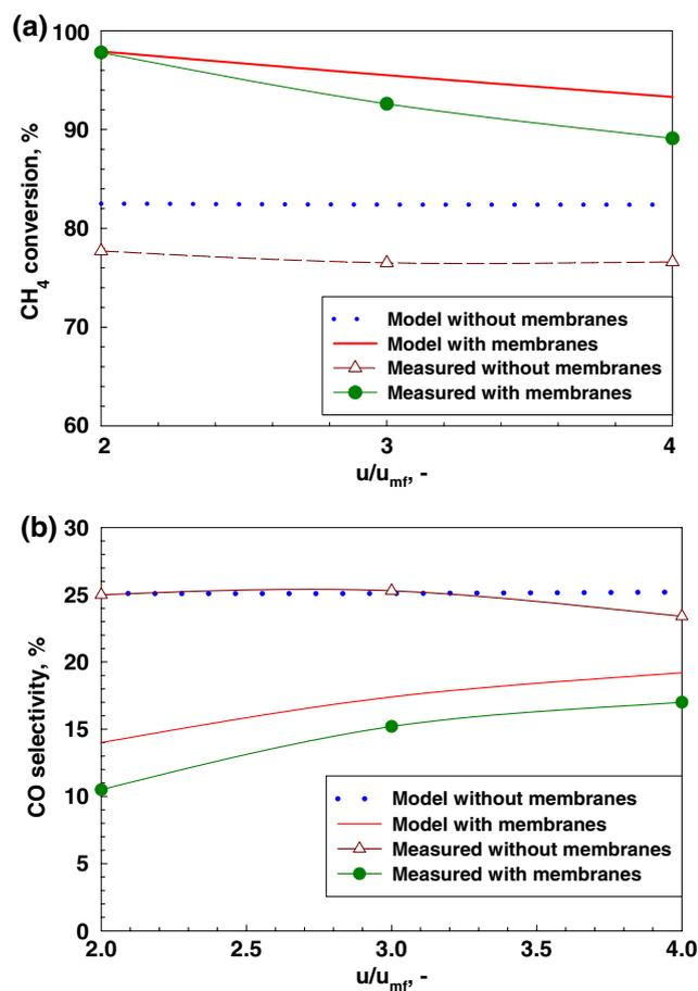
**Fig. 9** Measured and calculated CH<sub>4</sub> conversion (a) and CO selectivity (b) as a function of the relative superficial gas velocity ( $u/u_{mf}$ ) with and without membranes (methane combustion configuration,  $T = 600\text{ }^\circ\text{C}$ ,  $p = 2\text{ bar}$ ,  $u/u_{mf} = 2-4$ ,  $H_2O/CH_4 = 4$ ,  $O_2/CH_4 = 0.2$ )
