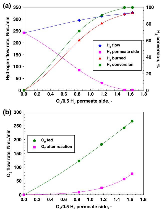
**Fig. 13** Results in case of oxidative sweeping for a feed of 35% H<sub>2</sub> at 500 °C ( $p = 3$  bar, sweep gas flow rate = 4.5 NL/min)
