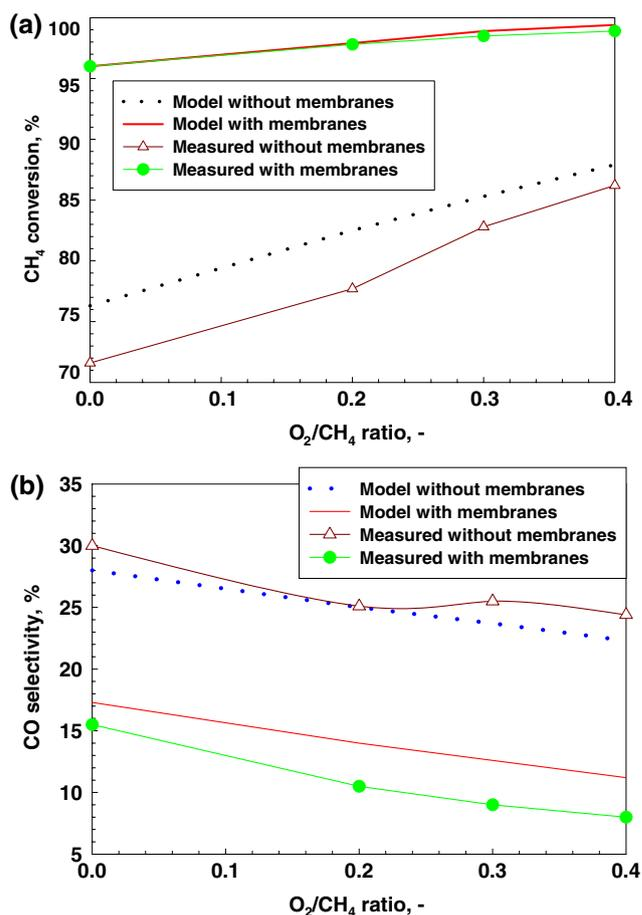
**Fig. 7** Measured and calculated CH<sub>4</sub> conversion (a) and CO selectivity (b) as a function of the O<sub>2</sub>/CH<sub>4</sub> ratio in the feed with and without membranes (methane combustion configuration,  $T = 600 \text{ °C}$ ,  $p = 2 \text{ bar}$ ,  $u/u_{mf} = 2$ ,  $\text{H}_2\text{O}/\text{CH}_4 = 4$ ,  $\text{O}_2/\text{CH}_4 = 0\text{--}0.4$ )
