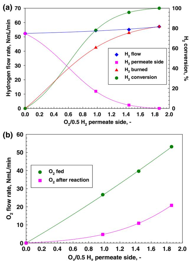
**Fig. 12** Results in case of oxidative sweeping for a feed of 5% H<sub>2</sub> at 500 °C ( $p = 3$  bar, sweep gas flow rate = 4.5 NL/min)
