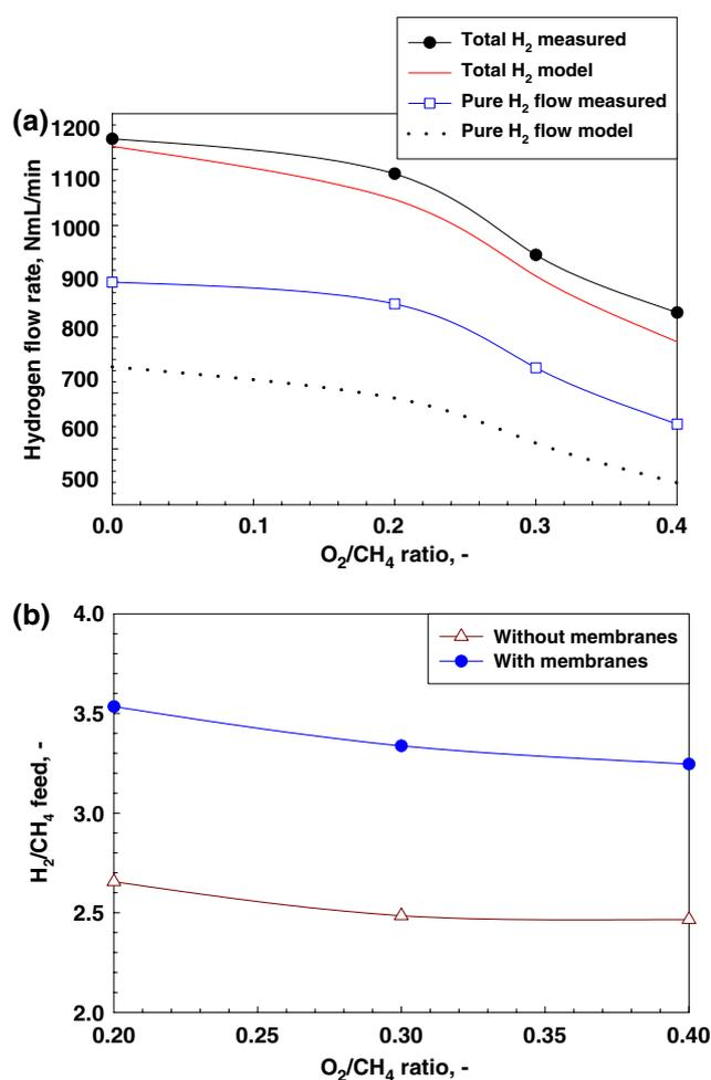
**Fig. 8** Measured and calculated total H<sub>2</sub> production and extracted H<sub>2</sub> flow rate (a) and H<sub>2</sub> yield (extracted H<sub>2</sub>/CH<sub>4</sub> fed) (b) as a function of the O<sub>2</sub>/CH<sub>4</sub> ratio in the feed (methane combustion configuration,  $T = 600$  °C,  $p = 2$  bar,  $u/u_{mf} = 2$ , H<sub>2</sub>O/CH<sub>4</sub> = 4)
