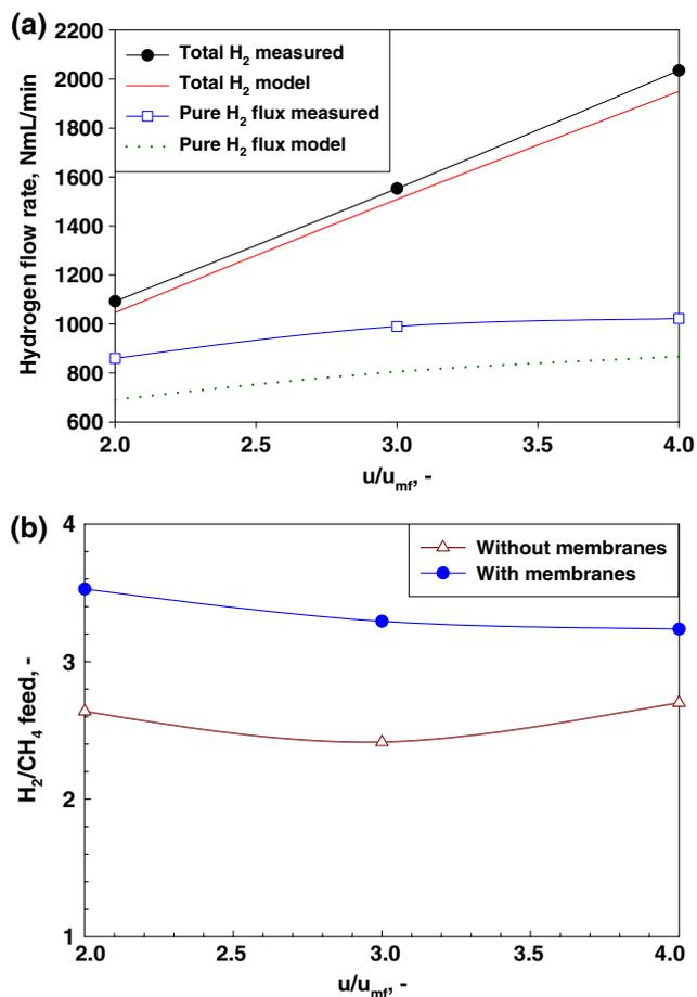
**Fig. 10** Measured and calculated total H<sub>2</sub> production and extracted H<sub>2</sub> flow rate (a) and H<sub>2</sub> yield (extracted H<sub>2</sub>/CH<sub>4</sub> fed) (b) as a function of the relative superficial gas velocity ( $u/u_{mf}$ ) (methane combustion configuration,  $T = 600\text{ }^\circ\text{C}$ ,  $p = 2\text{ bar}$ ,  $u/u_{mf} = 2$ ,  $H_2O/CH_4 = 4$ ,  $O_2/CH_4 = 0.2$ )
