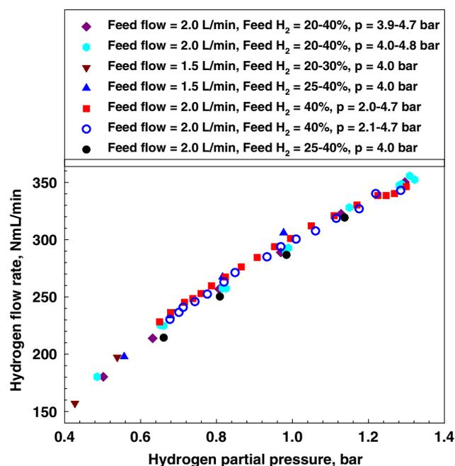
**Fig. 4** Hydrogen permeation flow rate through a U-shaped membrane as a function of the hydrogen partial pressure ( $T = 600\text{ }^{\circ}\text{C}$ )
