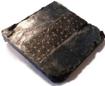
**Figure 1:** Picture of a specimen after squeezing. The dots on the surface were marked prior testing to determine whether the material slips at the walls.
