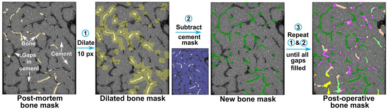
**Figure 2.** Segmentation procedure to obtain the post-operative bone mask from the post-mortem bone mask.
