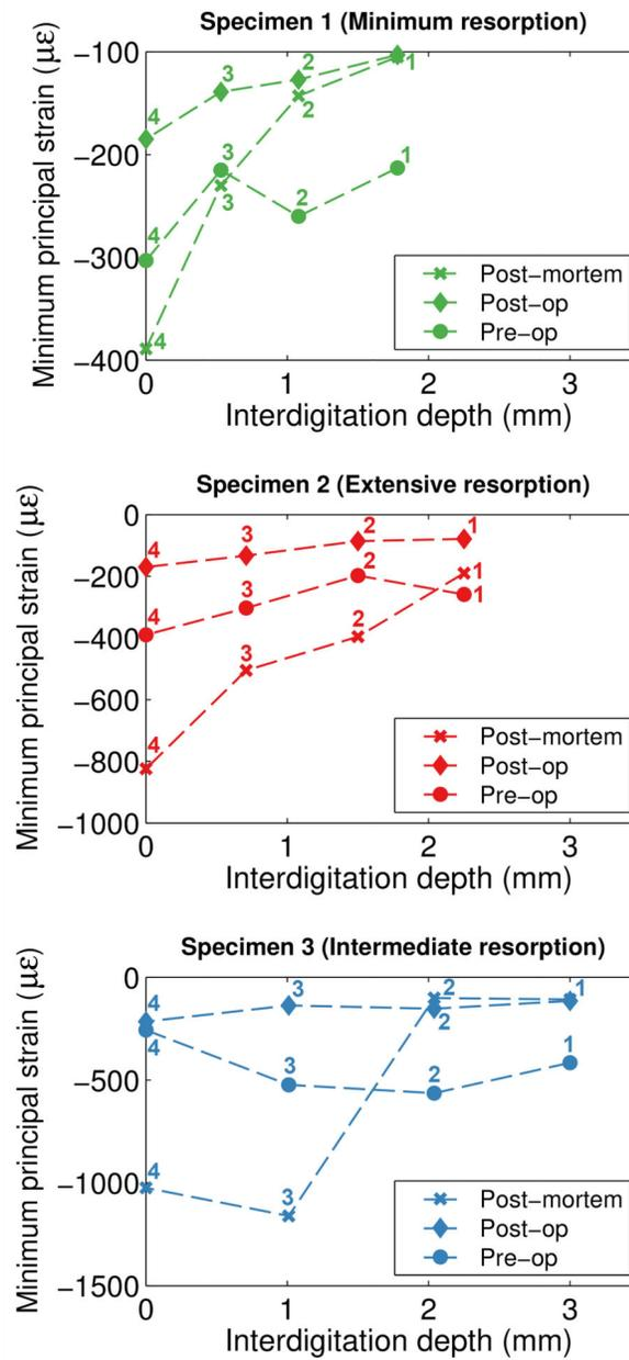
**Figure 7.** Interdigitated bone strain as a function of interdigitation depth shows a similar pattern for the FE models of all three specimens.
