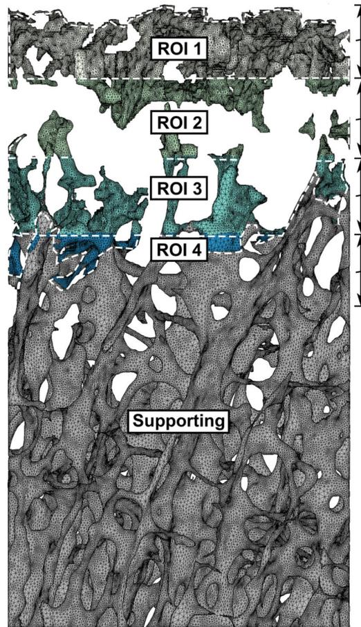
**Figure 5.** Post-mortem interdigitated bone for specimen 3 (intermediate resorption) with four regions of interest (ROI 1–4) having equal thickness. Supporting bone was chosen as the layer of bone immediately distal to the interdigitated bone.
