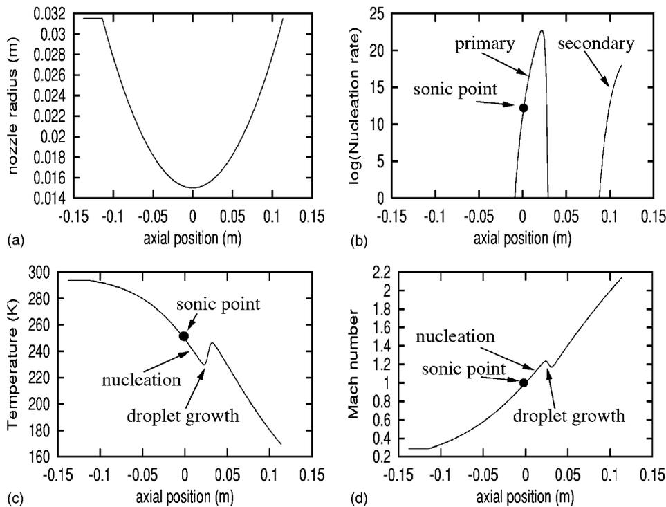
FIG. 1. Typical characteristics of condensing flow in a symmetric nozzle: (a) Nozzle radius, (b) nucleation rate, (c) temperature, and (d) Mach number.
