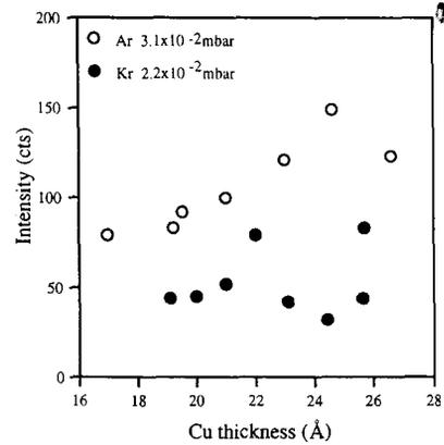
Fig. 3. A plot of (200) peak intensities as a function of Cu thickness for films sputtered with Kr and Ar. (The (111) peak shows similar behavior.)
