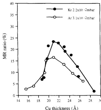
Fig. 1. MR ratio plotted as a function of Cu thickness for films sputtered with Kr and Ar.
