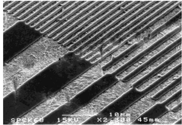
**Figure 1.** Scanning electron micrograph of four different microtextures on the cpTi wafer surfaces. The dents in the surface and consequential pattern damage are clearly visible. Furthermore, the protrusions on the surface edge and the difference in the roughness of the groove bottom and ridge crest can be seen.
