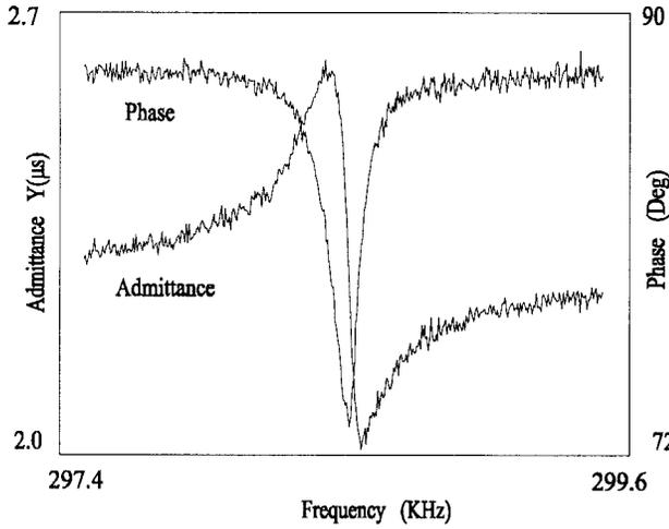
Fig. 5. Admittance, phase versus frequency plot (nonhysteresis). Resonator number is 3209, size is  $210 \times 100 \times 1.5 \mu\text{m}$ , gap spacing is  $1.0 \mu\text{m}$ ,  $V_p = 1 \text{ V}$ ,  $V_{\text{osc}} = 10 \text{ mV}$ , and  $Q_1 = 2871$ .
