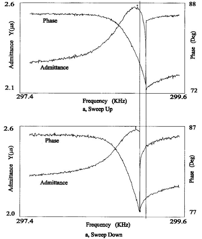
Fig. 7. Admittance, phase versus frequency plots (hysteresis). Top shows admittance and phase versus frequency plot for frequency sweep up. Bottom shows admittance and phase versus frequency plot for frequency sweep down. The hysteresis is clearly seen. Resonator number is 3209, size is  $210 \times 100 \times 1.5 \mu\text{m}$ , gap spacing is  $1.0 \mu\text{m}$ ,  $V_p = 1 \text{ V}$ ,  $V_{\text{osc}} = 20 \text{ mV}$ , and  $Q_1 = 2871$ .
