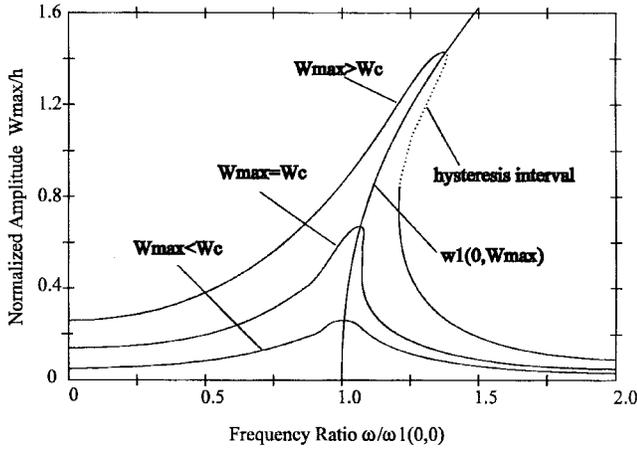
Fig. 2. Normalized amplitude versus the normalized frequency for a clamped-clamped beam with a rectangular cross section and with zero built-in axial strain [6].
