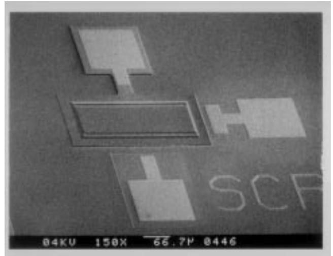
Fig. 4. An SEM photograph of cap and bond pads of the microbridge.
