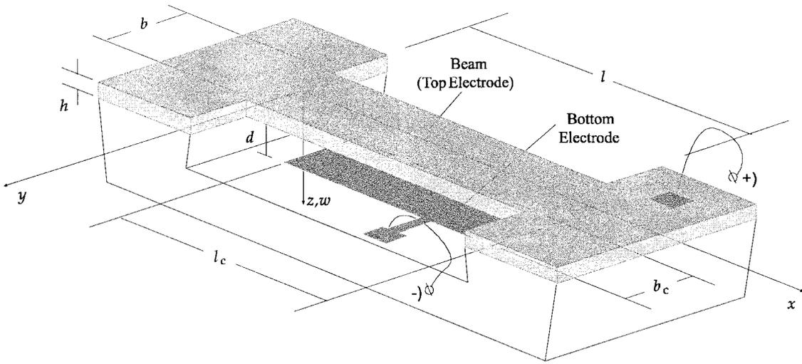
Fig. 1. Schematic drawing of a beam (length  $l$ , width  $b$ , and thickness  $h$ ) configured as a one-port resonator. The beam itself is homogeneous and is composed of a conducting material. The lower electrode considered here has the same shape as the beam (length  $l_c = l$  and width  $b_c = b$ ) [9].
