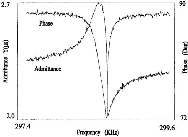
Fig. 6. Admittance, phase versus frequency plot (at critical load). Resonator number is 3209, size is  $210 \times 100 \times 1.5 \mu\text{m}$ , gap spacing is  $1.0 \mu\text{m}$ ,  $V_p = 1 \text{ V}$ ,  $V_{\text{osc}} = 15 \text{ mV}$ , and  $Q_1 = 2871$ .
