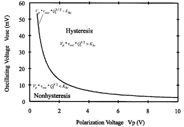
Fig. 3. Hysteresis criterion of a typical encapsulated LPCVD polysilicon resonant microbridge. The resonator size is  $210 \times 100 \times 1.5 \mu\text{m}$ . The gap spacing is  $1.0 \mu\text{m}$ , and the pull-in voltage is  $28.0 \text{ V}$ .  $Q_1 = 2700$ . The plate modulus  $E' = 166 \text{ GPa}$ , and a Poisson's ratio of  $0.22$  for the LPCVD polysilicon was used.
