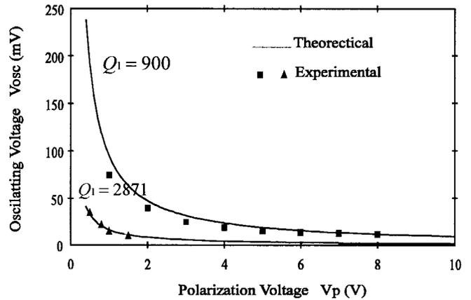
Fig. 8. Hysteresis criterion for resonator with a length of  $210 \mu\text{m}$ . Resonator size is  $210 \times 100 \times 1.5 \mu\text{m}$ . Resonator number is 3209,  $Q_1 = 2871$ , resonator number is 3220, and  $Q_1 = 900$ . The solid lines are the theoretical results calculated from (5). A plate modulus of 166 GPa and a Poisson’s ratio of 0.22 were used in the calculations. Higher quality factor means less freedom in choosing the driving voltages.
