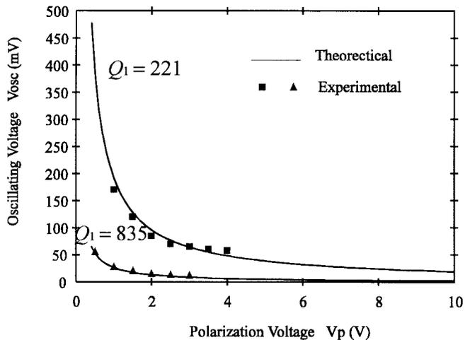
Fig. 9. Hysteresis criterion for resonator with a length of  $310\ \mu\text{m}$ . Resonator size is  $310 \times 100 \times 1.5\ \mu\text{m}$ , resonator number is 3304,  $Q_1 = 835$ , resonator number is 5307, and  $Q_1 = 221$ . The solid lines are the theoretical results calculated from (5). A plate modulus of 166 GPa and a Poisson's ratio of 0.22 were used in the calculations. Lower quality factor implies larger freedom in choosing the driving voltages.
