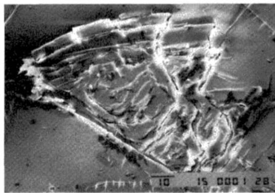
Fig. 3. SEM photograph of impact site on KAP(010). The contact caused partial removal of thin plates from the surface, probably due to (010) being a cleavage plane. The thin black bar denotes 10  $\mu\text{m}$ .
