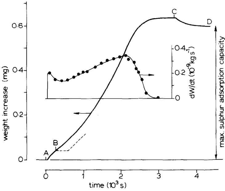
Figure 2 Typical weight registration of sulphur accumulation NaY(2.40) zeolite, 1.65 mg, 188 °C.
