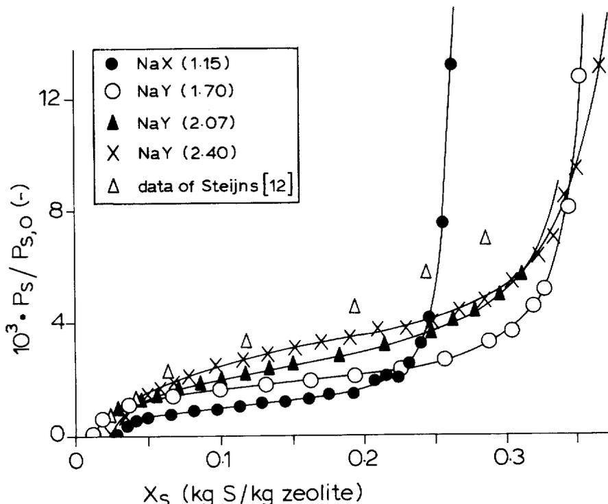
Figure 9 Relative sulphur vapour pressure for desorption of sulphur from NaX and NaY zeolites.
