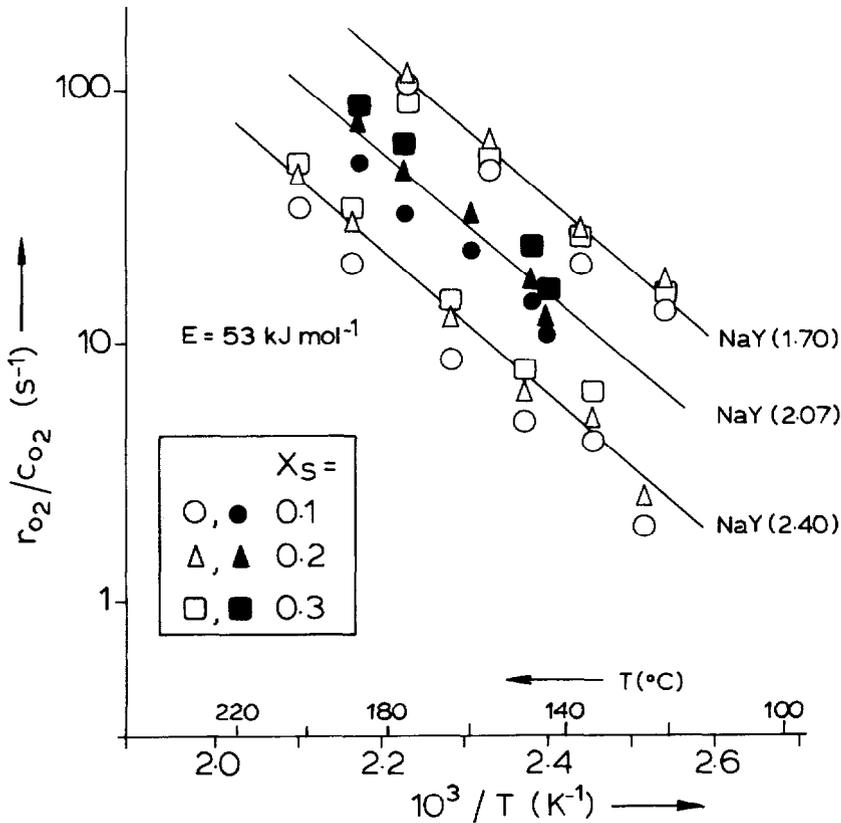
Figure 7 Arrhenius plot of reaction rate constants.
