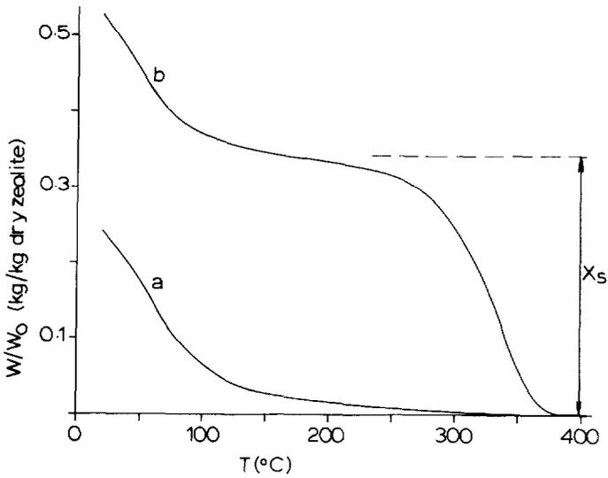
Figure 3 Thermoanalysis of NaY(2.40) (1.65 mg, heating rate  $0.17 \text{ }^\circ\text{C s}^{-1}$ ). (a) fresh. (b) containing 0.34 kg sulphur per kg dry zeolite.
