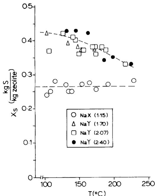
Figure 4 Maximum sulphur adsorption capacity of NaX and NaY zeolites versus temperature.
