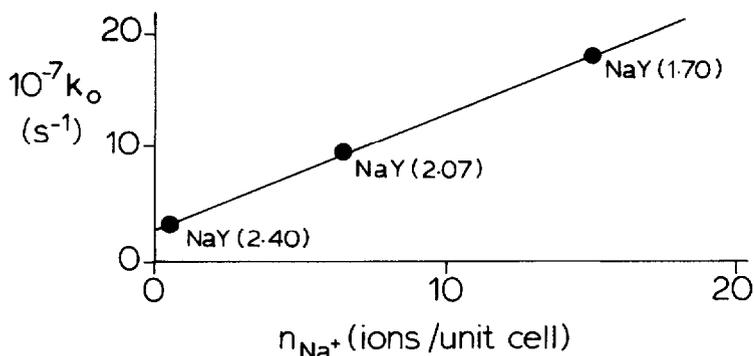
Figure 8 Frequency factors of the Arrhenius equation versus the calculated  $Na^+$  concentration in the supercages.
