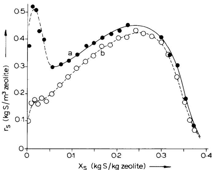
Figure 5 Reaction rate of the oxidation of  $\text{H}_2\text{S}$  with  $\text{O}_2$  versus the sulphur load (zeolite NaY(1.70), 150 °C)(a) first experiment (b) fourth experiment.
