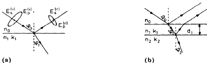
Fig. 6 Schematic representation of the reflection of polarized light. (a) Clean surface, (b) surface covered with single layer.
