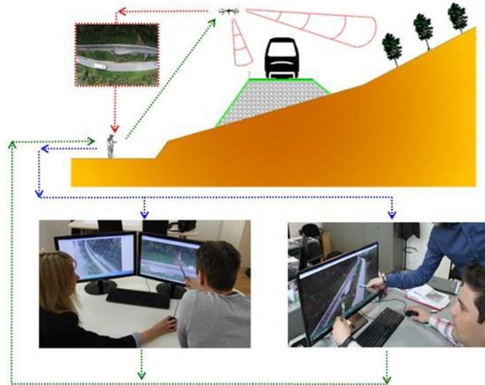
Fig. 4. Interactive procedure of visual assessment using UAV.
