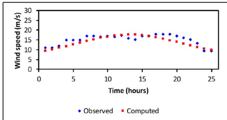
Figure 5. Observed and computed wind speed for the storm at March 1, 2008.
