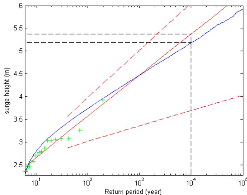
**Figure 8. Surge levels based on model output are denoted in blue. Statistical extrapolation based on extrapolation of measurements (green plusses) is shown by the solid red line. The corresponding 95% probability interval is shown by red dashed lines.**
