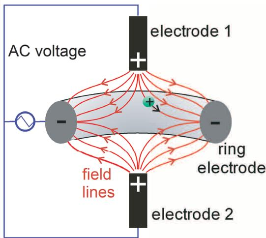
FIGURE 4: (left) Demonstration model of a Paul trap with a grain of milk powder caught in the center of the high-voltage electrodes. (right) Instantaneous electric field lines in the trap showing the direction in which a positively charged particle would fly. Before the particle hits an electrode, though, the polarity is flipped. This AC electric field causes a micromotion effectively trapping the particle in the center of the trap.
