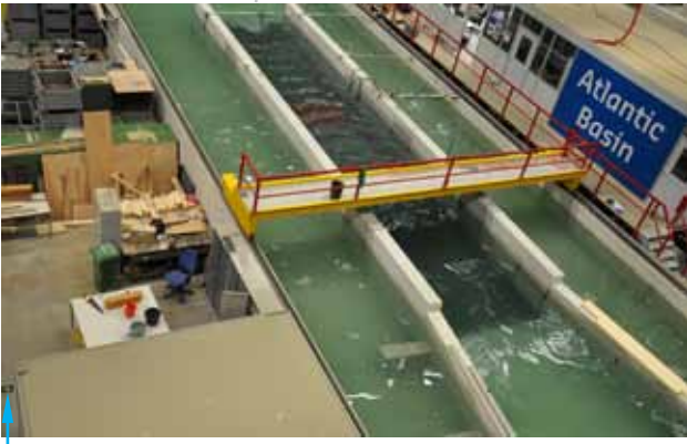
FIG. 4 Illustration of the experimental facility at Deltares. Flow is from bottom to top. The measurements were carried out at the end of the concrete channel.
