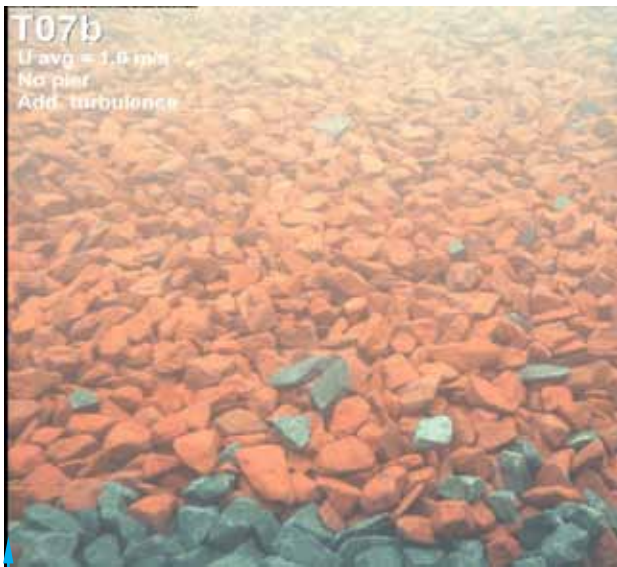
FIG. 6 Single images (also see FIG. 7) of cameras that were used to determine bed and filter movement during the test. Camera on test section 1 without pier
