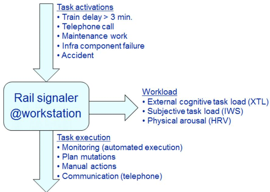
Figure 2 Task flow of a rail signaller at their workstation
