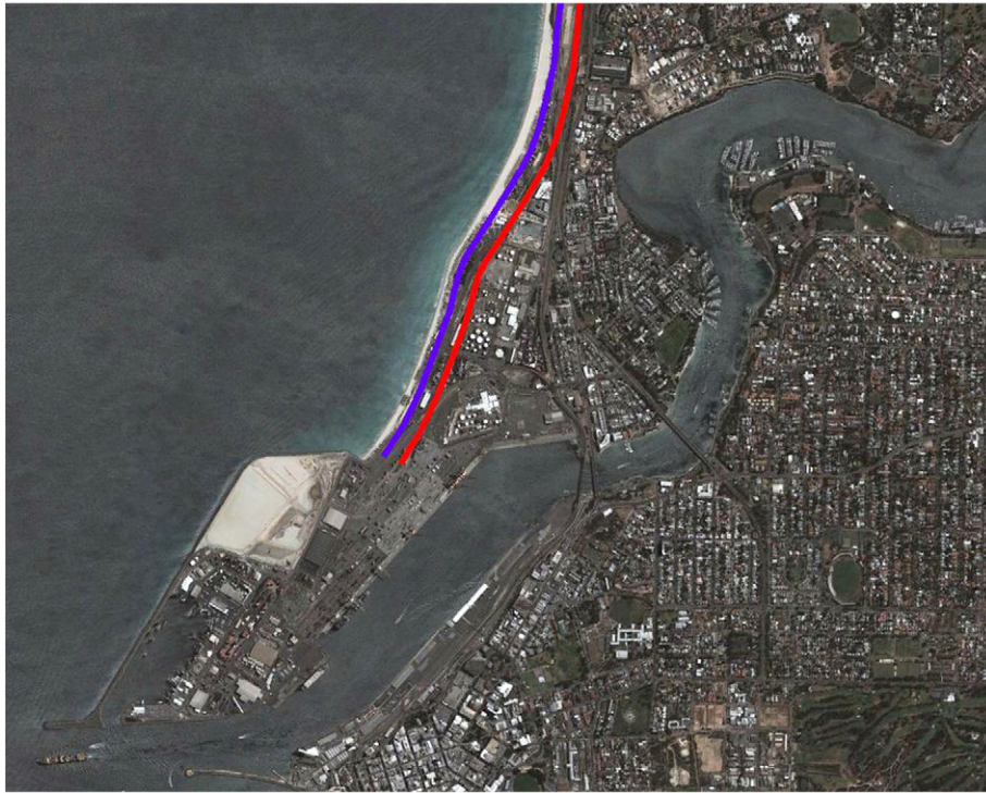
Fig. 4. SMIC Model predicted coastline change at Swan River inlet, Australia by 2100 (red line) and coastline change due to the Bruun effect alone (blue line) (after Ranasinghe et al., 2013).
