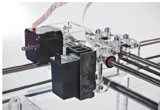
Figure 3 X-gantry with attached Hewlett-Packard C6602A cartridge and roller
