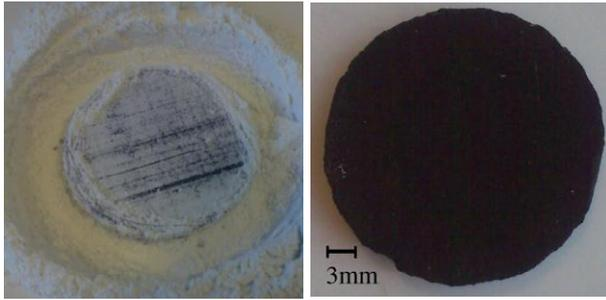
Figure 4 (left) Green gypsum part is excavated in powder bed and (right) fixated gypsum part (diameter 28mm)
