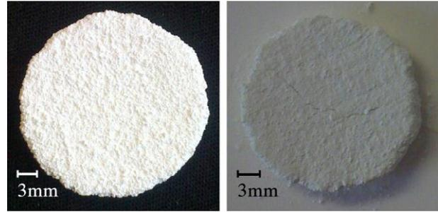
Figure 5 (left) Sintered alumina part (diameter 27mm) (right) sintered alumina-zirconia part (diameter 23mm)
