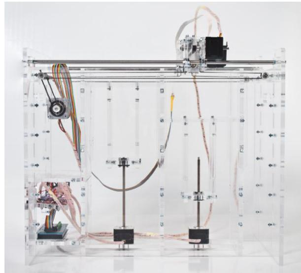
Figure 2 The machine from in profile. Electronics compartment bottom left. Y-stepper top left. Linear position drives and pistons centre and X-gantry top right.
