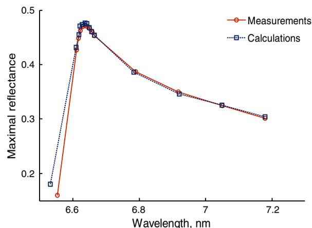
**Fig. 3** Measured and fitted peak reflectivity for a 150 period LaN/B<sub>4</sub>C multilayer mirror. The mirror had a lateral gradient in periodicity. The data points represent the maximum reflectance and corresponding wavelength at various positions on the mirror.
