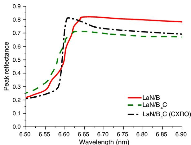
**Fig. 1** Peak reflectivity of a perfect LaN/B multilayer mirror calculated using measured B optical constants (16) (line) and a LaN/B<sub>4</sub>C multilayer mirror calculated using measured (17) (dashed) and Henke (13) (dashed-dotted) optical constants.
