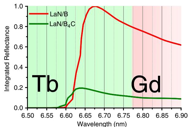
**Fig. 2** Normalized integrated reflectivity for a 10-element mirror system consisting of LaN/B (red) and LaN/B<sub>4</sub>C (green) multilayer mirrors, as calculated using measured optical constants for B (16) and B<sub>4</sub>C (17). The region of the Tb radiation spectrum is indicated with a green background and of Gd with a red background (12).
