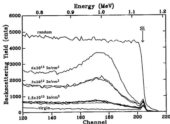
FIG. 1. Si portion of RBS/channeling spectra following In implantations. The single  $6 \times 10^{13}$  1.0 MeV In/cm<sup>2</sup> implant (samples 1 and 2) leads to a high level of damage and each  $3 \times 10^{13}$  In/cm<sup>2</sup> implant for sample 3 results in an intermediate level of damage. For sample 4, each  $1.5 \times 10^{13}$  In/cm<sup>2</sup> implant only causes a low amount of damage. Random and channelled spectra of virgin Si(100) are also shown.
