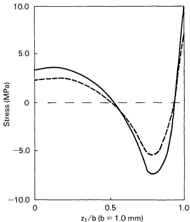
Fig. 8b. Stress distribution for segment 2. Solid line: series No23. Dashed line: series No23+.
