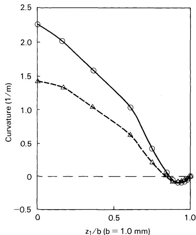
Fig. 8a. Curvature of segment 2 as a function of dimensionless coordinate  $z_1/b$ . Solid line: series No23.  $\circ$ : data point. Dashed line: series No23+.  $\Delta$ : data point.
