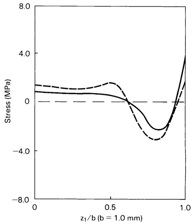
Fig. 10b. Stress distribution for series PS55. Solid line: beginning of flow path (segment 1). Dashed line: end of flow path (segment 3).
