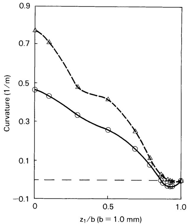
Fig. 10a. Curvature as a function of dimensionless coordinate  $z_1/b$  for series PS55. Solid line: beginning of flow path (segment 1).  $\circ$ : data point. Dashed line: end of flow path (segment 3).  $\Delta$ : data point.
