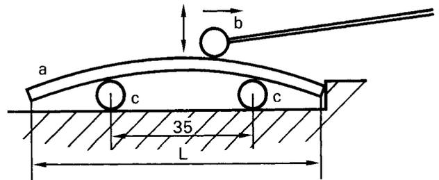
Fig. 2. Configuration for deflection measurement. Layers are successively removed from the lower surface of the specimen. a: specimen; b: mechanical sensor; c: steel rod. L: length of chord.
