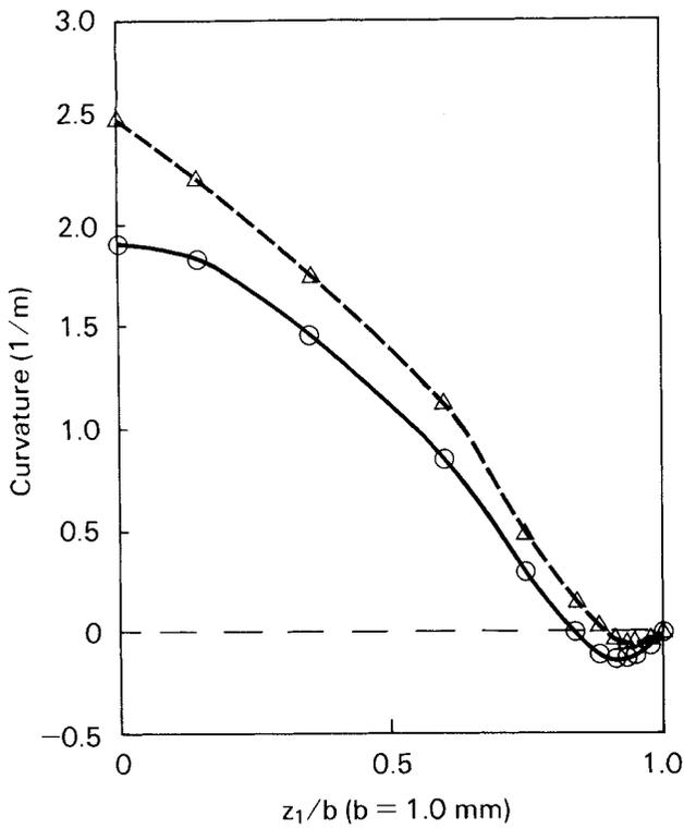
Fig. 11a. Curvature as a function of dimensionless coordinate  $z_1/b$  for series No23. Solid line: beginning of flow path (segment 1).  $\circ$ : data point. Dashed line: end of flow path (segment 3).  $\triangle$ : data point.
