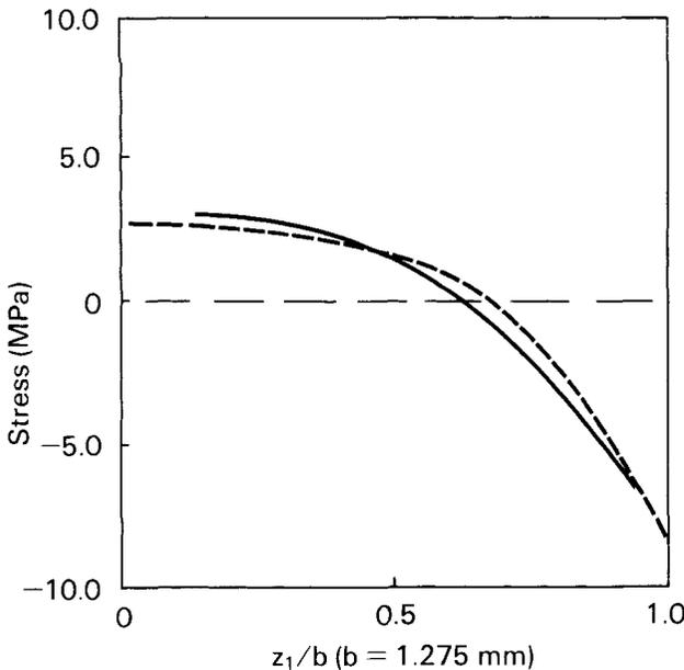
Fig. 4. Stress distributions of free-quenched compression-molded PS plates. Solid line: results of the present investigation. Dashed line: results of Isayev (12). Position  $z_1/b = 0$ : original center plane of specimen. Position  $z_1/b = 1$ : original surface plane of specimen.
