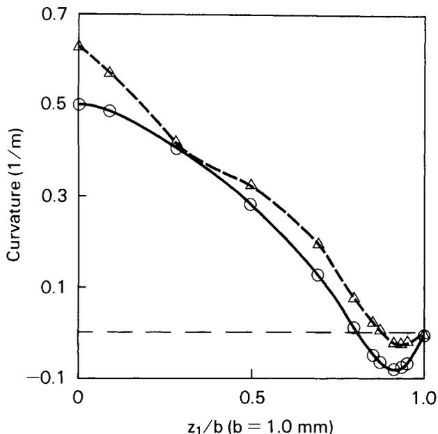
Fig. 7a. Curvature of segment 2 as a function of dimensionless coordinate  $z_1/b$ . Solid line: series PS25. ○: data point. Dashed line: series PS55. △: data point.
