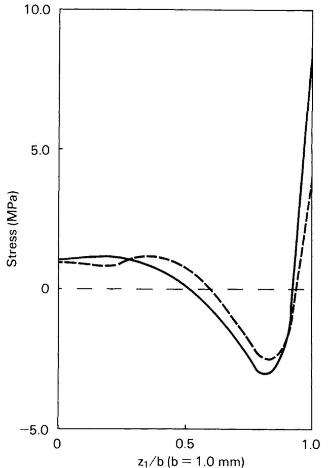
Fig. 7b. Stress distribution for segment 2. Solid line: series PS25. Dashed line: series PS55.
