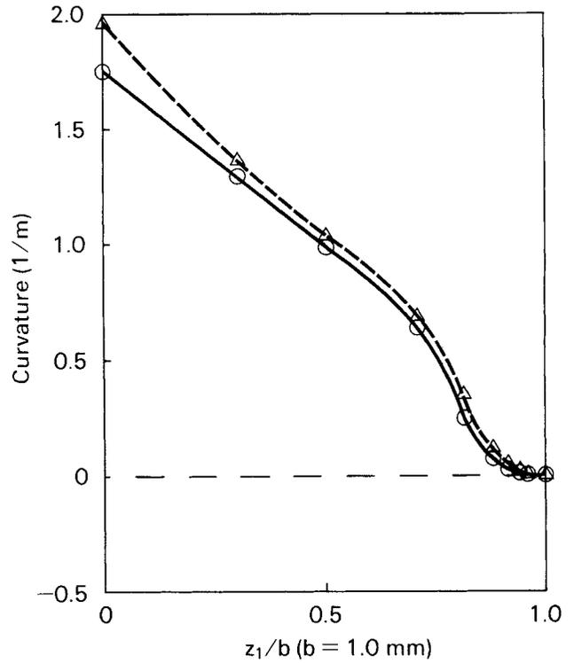
Fig. 12a. Curvature as a function of dimensionless coordinate  $z_1/b$  for series PC50. Solid line: beginning of flow path (segment 1).  $\circ$ : data point. Dashed line: end of flow path (segment 3).  $\triangle$ : data point.
