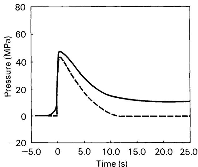
Fig. 9a. Pressure profiles for series PS55. Solid line: pressure at P3. Dashed line: pressure at P4.
