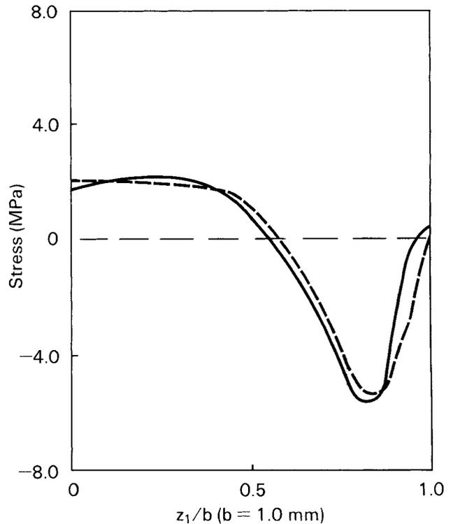
Fig. 12b. Stress distribution for series PC50. Solid line: beginning of flow path (segment 1). Dashed line: end of flow path (segment 3).
