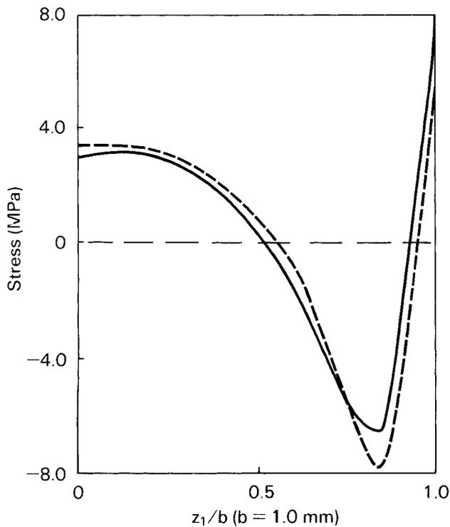
Fig. 11b. Stress distribution for series No23. Solid line: beginning of flow path (segment 1). Dashed line: end of flow path (segment 3).
