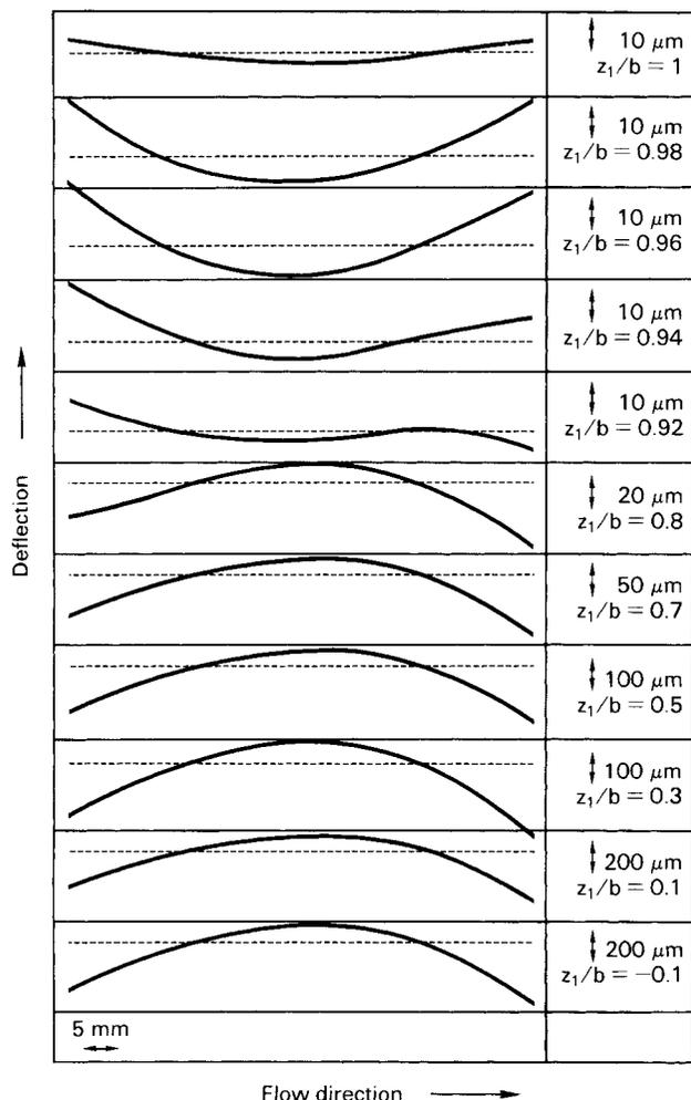
Fig. 5. Survey of deflection profiles of series PS55. Dashed line: reference line at arbitrary position.
