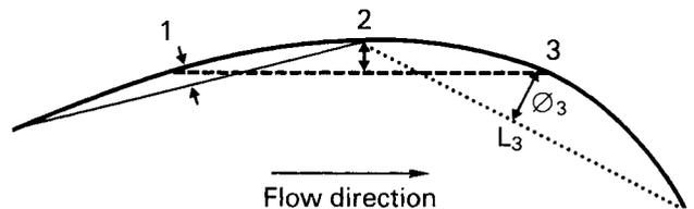
Fig. 3. Typical example of measured deflection profile, divided into 3 segments. Solid line: chord of segment 1. Dashed line: chord of segment 2. Dotted line: chord of segment 3.  $\phi_3$ : deflection for segment 3.  $L_3$ : length of chord for segment 3.
