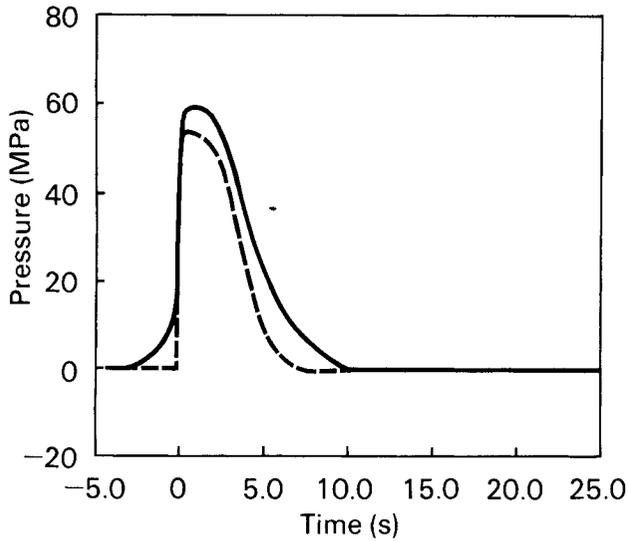
Fig. 9b. Pressure profiles for series No23. Solid line: pressure at P3. Dashed line: pressure at P4.
