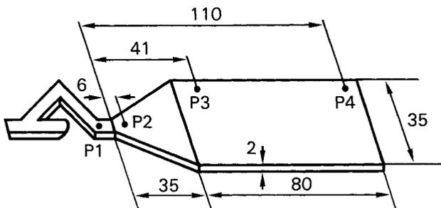
Fig. 1. Flat-plate configuration and location of pressure transducers P1 to P4 (dimensions in mm). The first (P1) is located at the end of the runner; the other transducers (P2, P3, P4) are located downstream from the entrance of the plate.
