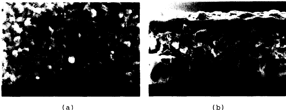
FIG. 3 Micrograph of SLM layer B: (a) top view; (b) cross section.
