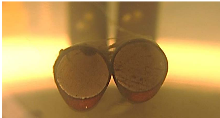
Figure 4-2: Working electrodes after 23 days of exposure.
