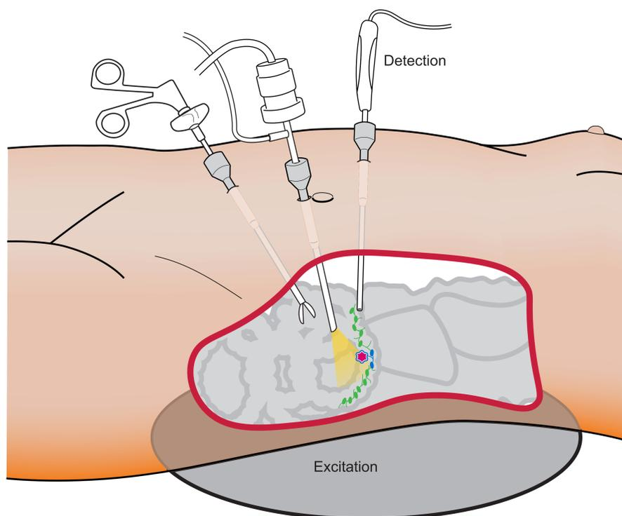
Figure 1 - Laparoscopic detection of sentinel lymph nodes using our DiffMag technique with separated excitation and detection coils.
