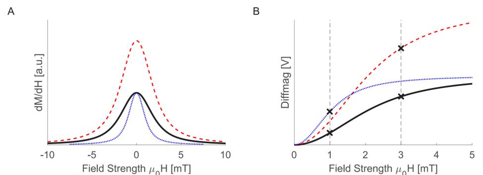
Figure 3 - Important characteristics of the magnetization curve to increase the DiffMag value. A) shows a fictional curve with an increased susceptibility (red) and one with a smaller field of saturation magnetization (blue) compared to the black curve. B) shows the corresponding DiffMag values.
