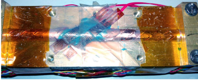
Fig. 5. Two flexible MINCO heaters are glued to two tapes for heating and introducing a normal zone.
