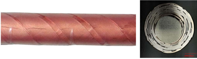
Fig. 1. (Left) CORC cable side view. (Right) Cross-sectional view of the CORC cable with 12 ReBCO layers.
