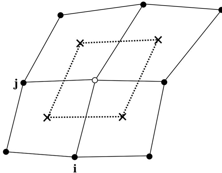
Figure 2: Control volume in the vertex-based method.
