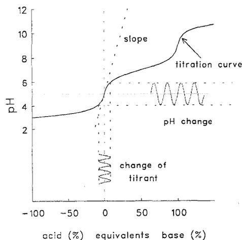
**Fig.2** Illustration of buffer capacity measurement by means of an applied sinusoidal perturbation of titrant.
