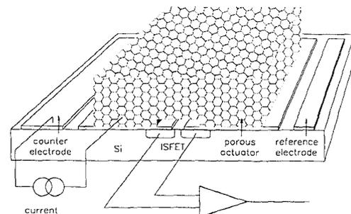
Fig.1 ISFET with a porous electrode covering the gate.
