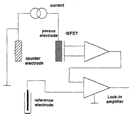
**Fig.3** Measurement set-up.
