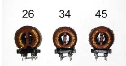
Fig. 4: The measured chokes with data-sheet values: 5 mH, 10 mH and 20 mH and their amount of turns from left to right. The core material is MnZn.
