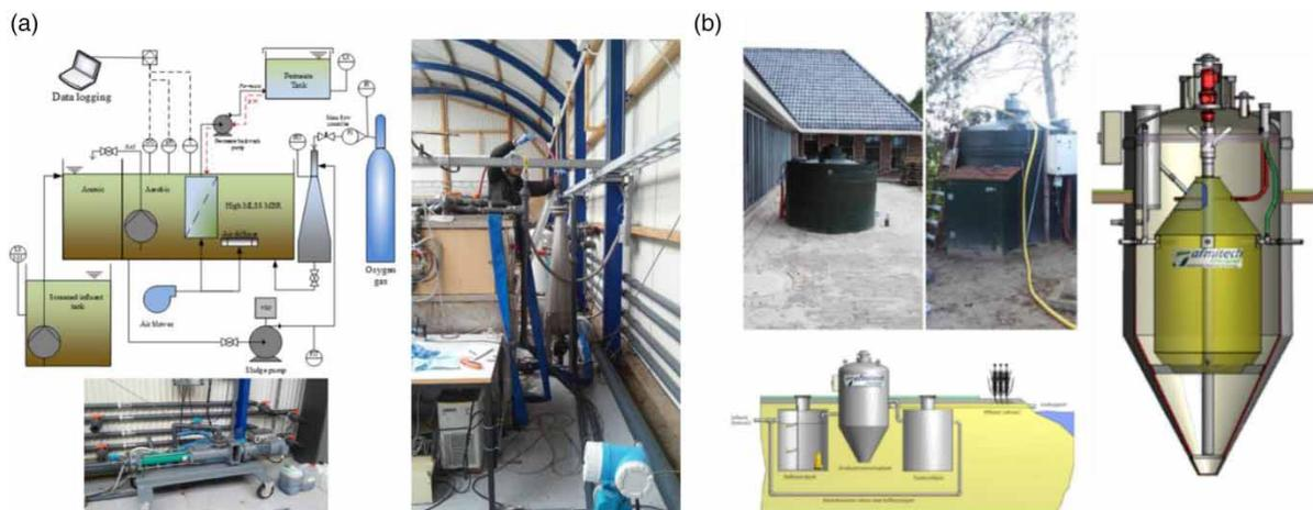
**Figure 1** | (a) Schematic process flow diagram and pictures of the installed prototype MBR setup in Delft, the Netherlands; (b) decentralized wastewater treatment system Bever III from the company Afmitech in Friesland, the Netherlands.
