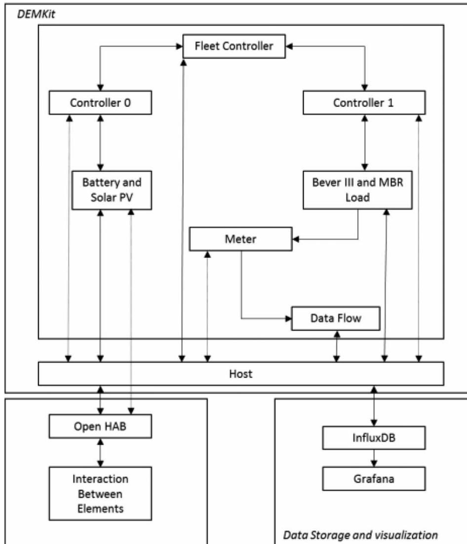
**Figure 2** | Diagram of the DEMKit platform with a model and external software.
