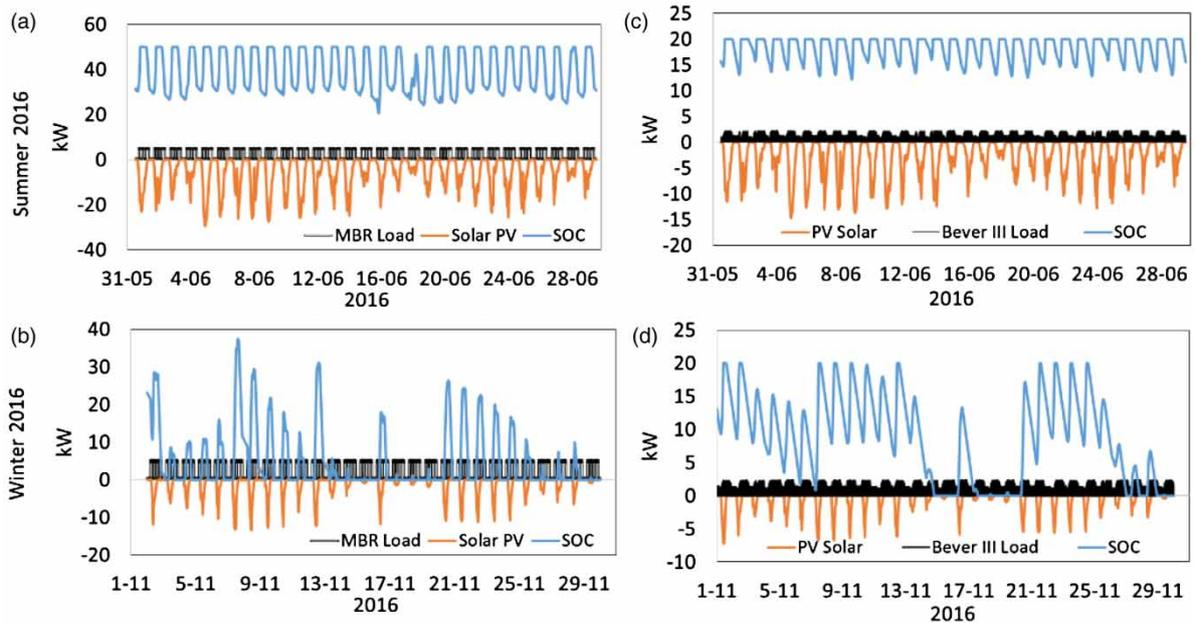
**Figure 3** | Energy profiles of the DWWTW using solar PV and the Sea-Salt battery in a 100% off-grid scenario: (a) MBR during June 2016; (b) MBR during November 2016; (c) Bever III during June 2016; and (d) Bever III during November 2016.
