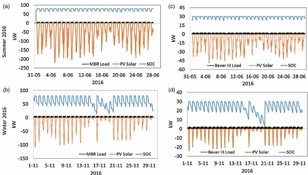
**Figure 4** | Oversized energy profiles for the DWWTW using solar PV and the Sea-Salt battery in a 100% off-grid scenario: (a) MBR during June 2016; (b) MBR during November 2016; (c) Bever III during June 2016; and (d) Bever III during November 2016.
