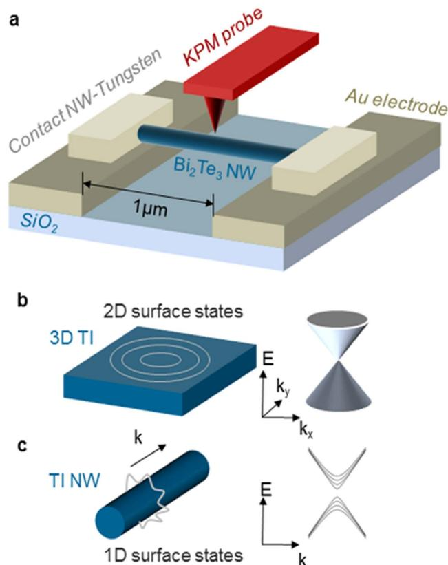
**Figure 1.** (a) Schematic diagram of the measurement set-up. (b) 3D topological insulators (TIs) exhibit 2D surface states, forming a Dirac cone. (c) TI nanowires exhibit 1D subbands on the surface, due to the quantum confined boundary condition along the perimeter direction.
