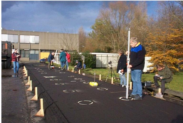
Figure 4: All measurements (temperature, level and rod, Strato test and Troxler) in progress.
