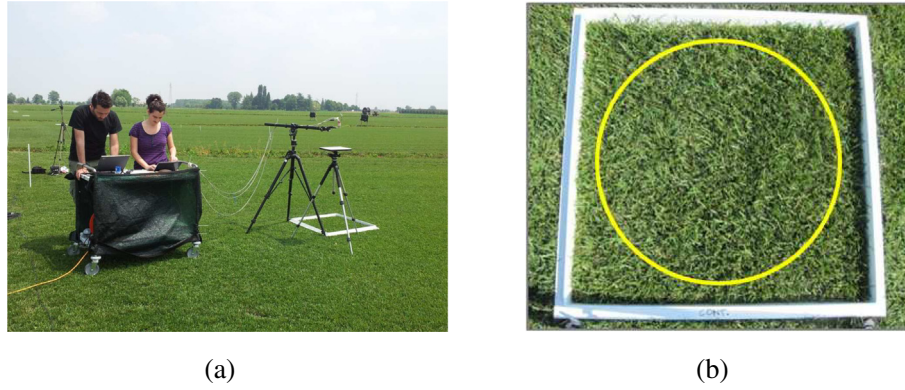
Fig. 1. a) Picture of the spectroscopic setup in the field; b) Parcel of the measured lawn: the yellow circle is approximately the area measured with the spectroscopic system. (For interpretation of the references to color in this figure legend, the reader is referred to the web version of this article.)
